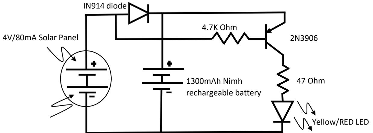
To perform the switching, we use a PNP transistor that is controlled by the voltage output from the solar panel. When it's sunny or there is enough light, the output of the panel is high, which turns off the transistor, but when it gets dark, the transistor lets current flow to our yellow/RED LED. This circuit works very well and is entertaining for students to learn the concepts. Pictures are shown below on the next page:
