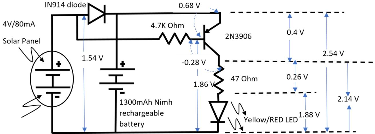
Voltage Levels When the LEDs are not glowing are shown in the figure below:
