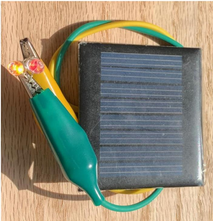
In the above picture, we have connected one of the panels directly to 2 LEDs, yellow and red. Be careful about the current rating of the solar panel and the LEDs. A “regular” LED designed for 20 mA can be destroyed by the current produced by the solar panel.
