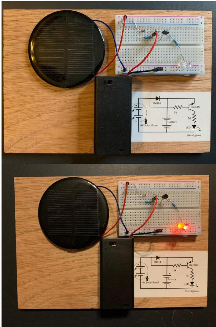
In the first picture, when there is enough light falling on the solar panel, LEDs are not glowing but instead the batteries are getting charged. This happens because the voltage generated in the solar panel due to the intensity of the light is switching off the PNP transistor 2N3906 and current can not flow through the LED. In the second picture when the light intensity is reduced, the LEDs start glowing because the PNP transistor 2N3906 switches on and current starts flowing through the LEDs.
