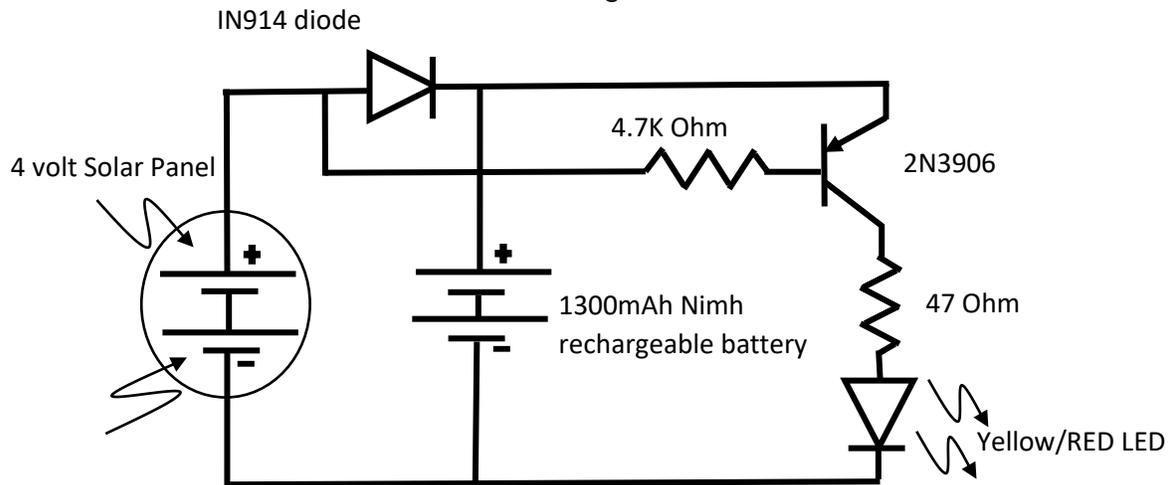
To perform the switching, we use a PNP transistor that is controlled by the voltage output from the solar panel. When it's sunny or there is enough light, the output of the panel is high, which turns off the transistor, but when it gets dark, the transistor lets current flow to our yellow/RED LED. This circuit works very well and is entertaining for students to learn the concepts.
